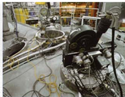
Figure 23 Fermilab bubble chamber: 4.6 m in diameter in a 3 T magnetic field
