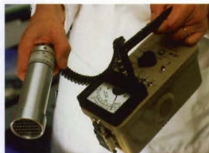
Figure 24 Geiger counter and GM tube
