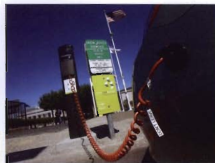
Figure 3 This plug-in Toyota Prius routinely gets more than 130 mpg. The black circle on the left of the back bumper is a plug socket, allowing an easy connection to the ac mains electrical supply.
