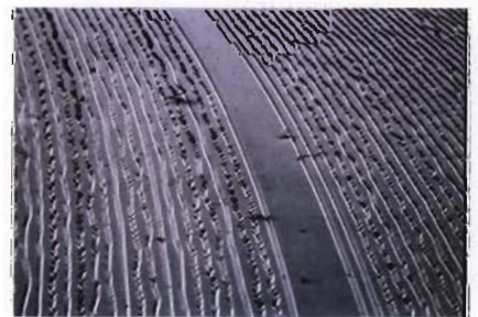
Figure 8 Magnified view of grooves in an LP record
