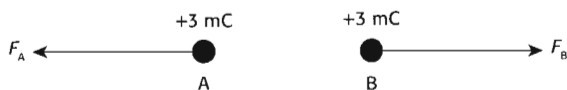
Figure 9 Each charge is +3 mC and neither one is free to move. The forces are equal and opposite.
